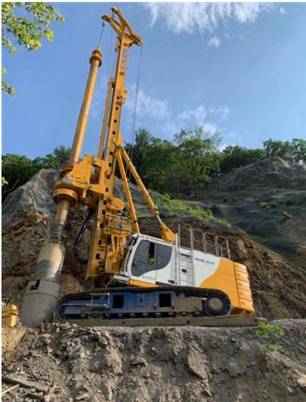
BAUER BG 26 rotary drilling rig
